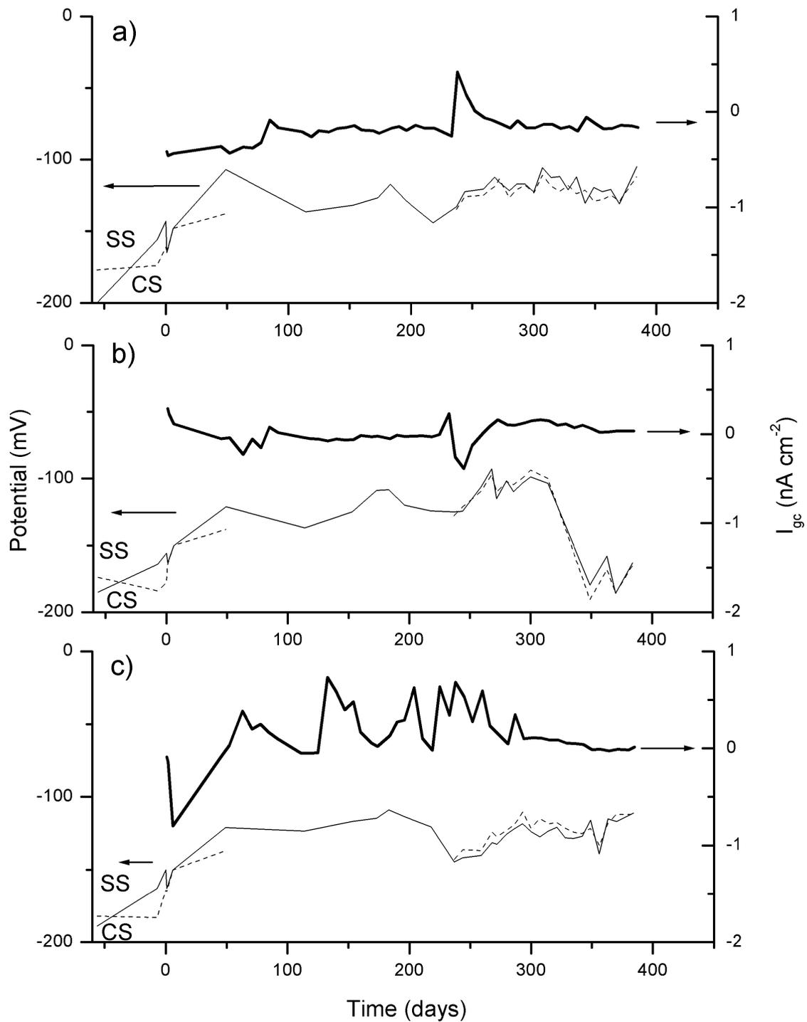
Figure 13. Galvanic coupling potentials and current densities measured in concrete specimens coupled by passive CS in chloride free environment with SSs in 3.5% Cl<sup>-</sup>: a) 2205; b) 304LN; c) 316LN.
