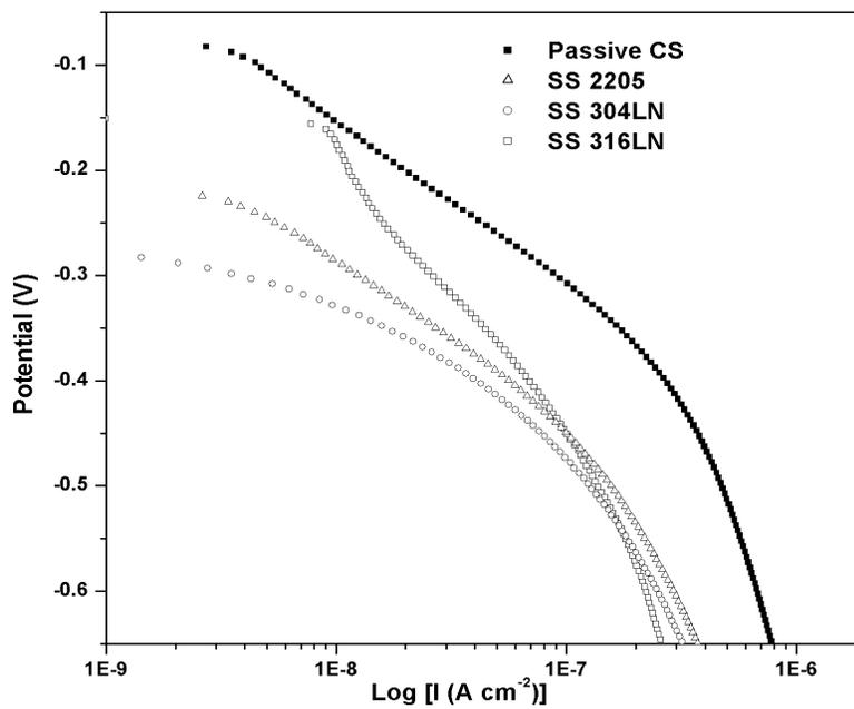
Figure 8. Cathodic polarization curves of passive CS and SS measured in a saturated  $\text{Ca}(\text{OH})_2$  solution.
