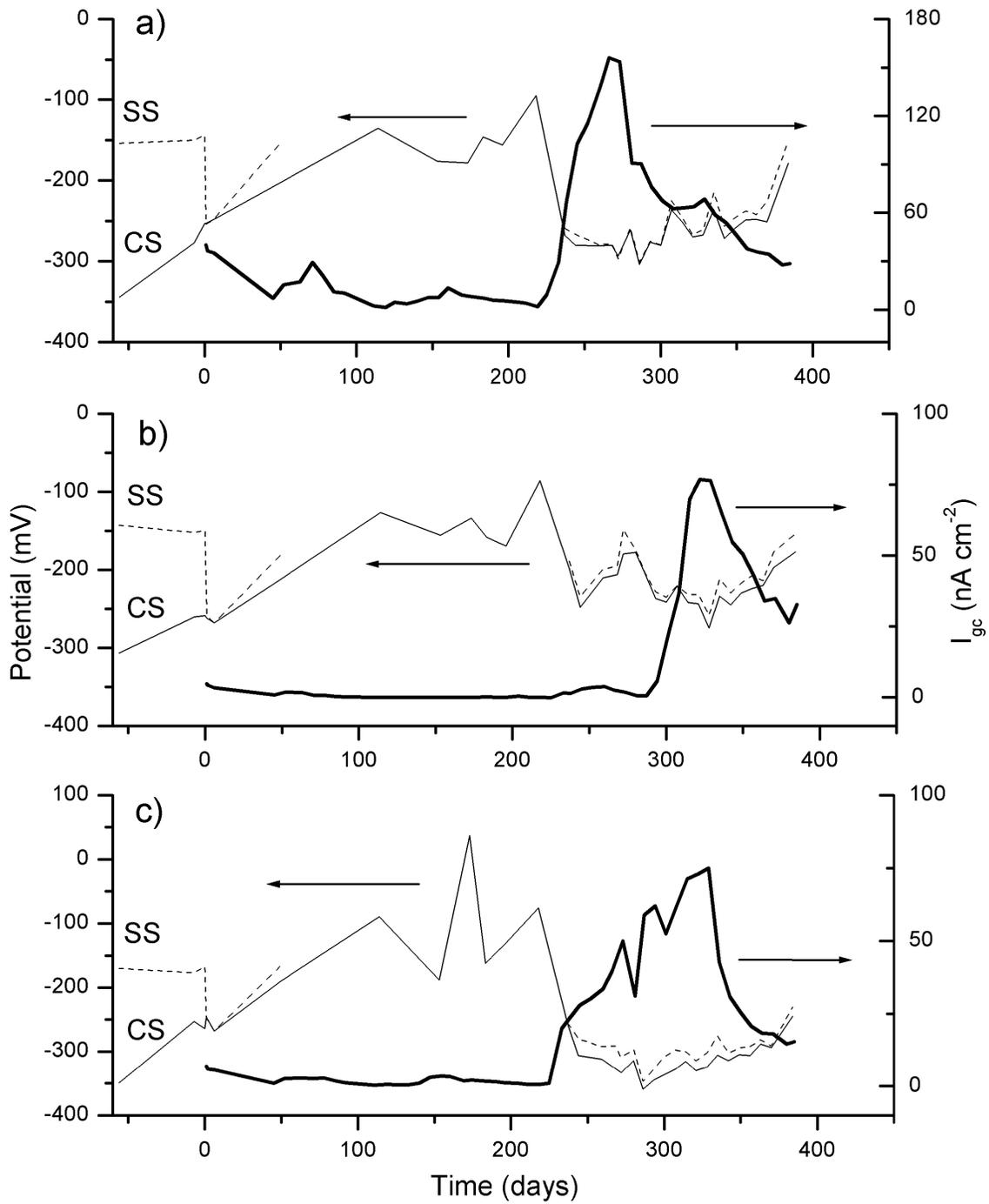
Figure 9. Galvanic coupling potentials and current densities measured in concrete specimens coupled by CS in 1.5% Cl<sup>-</sup> with SSs in a chloride free environment: a) 2205; b) 304LN; c) 316LN.
