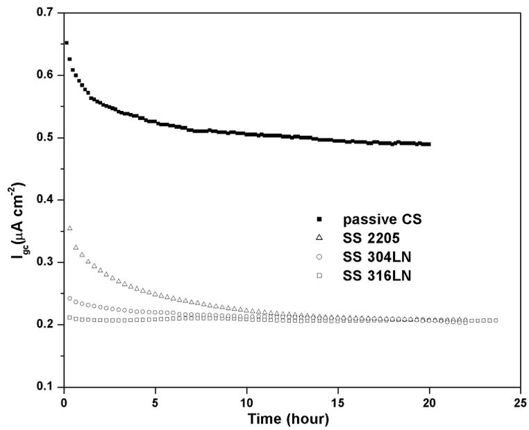
Figure 4. Curves of  $I_{gc}$  obtained by coupling corroding CS with passive CS or SSs 2205, 304LN and 316LN in a Saturated  $\text{Ca}(\text{OH})_2$  solution.
