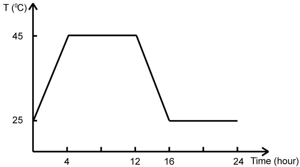
Figure 2. Temperature cycles controlled in environmental chamber.
