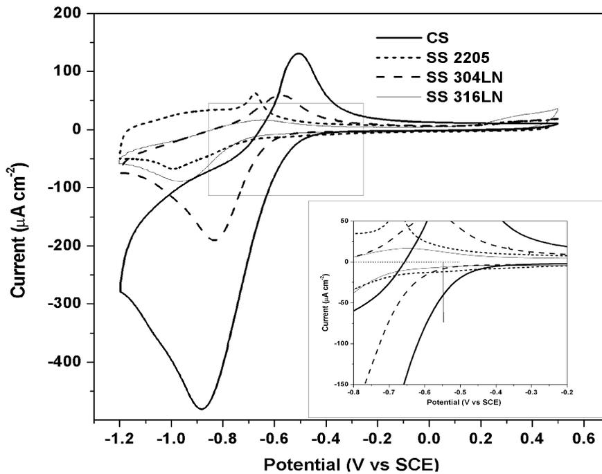
Figure 6. Cyclic voltammograms of passive CS and SS measured in a saturated  $\text{Ca}(\text{OH})_2$  solution (the inset shows the enlarged current scale).
