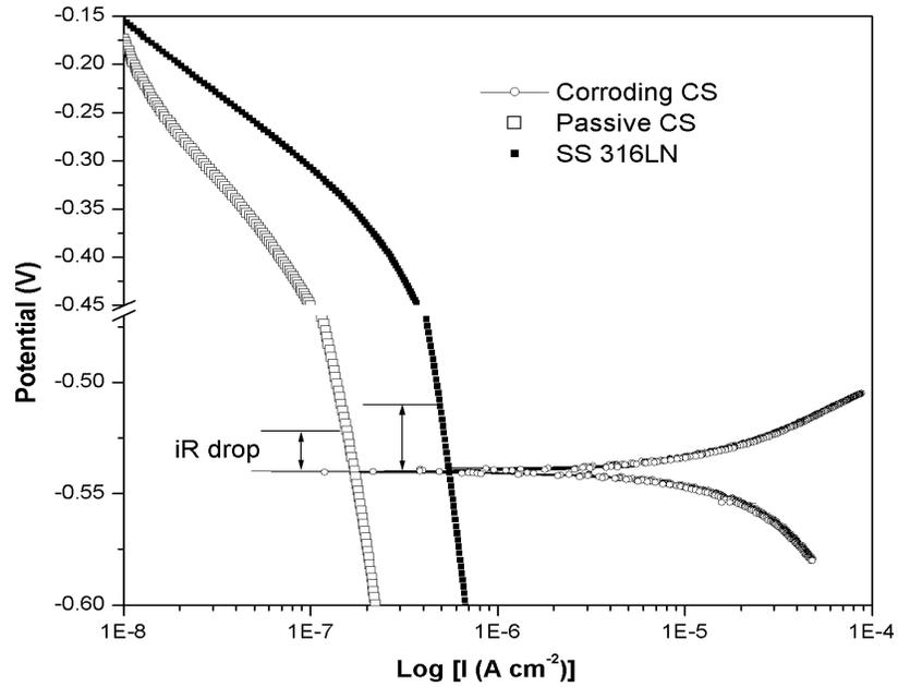
Figure 5. Polarization curves of corroding CS, passive CS and SS 316LN measured in a saturated  $\text{Ca}(\text{OH})_2$  solution.
