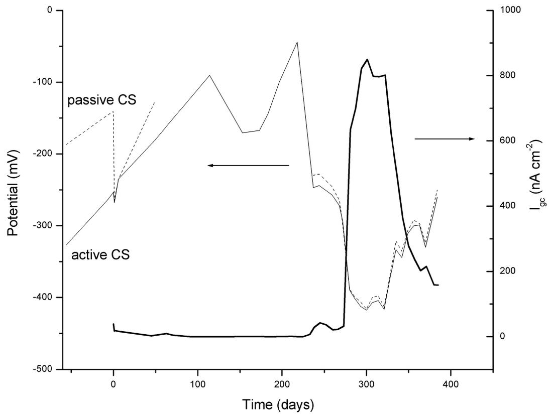
Figure 11. Galvanic coupling potentials and current densities measured in concrete specimens coupled by CS in 1.5% Cl<sup>-</sup> with passive CS in chloride free environment.
